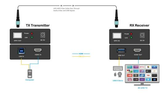
needed, this saves time and cost. Now a fiber optic connection can be made fast and reliable. Using the MPO connector on each end of the Celerity fiber optic cable, a secure snap-lock connection is made to the UFO-GTW-RED-4K-TX and UFO-GTW-RED-4K-RX.
